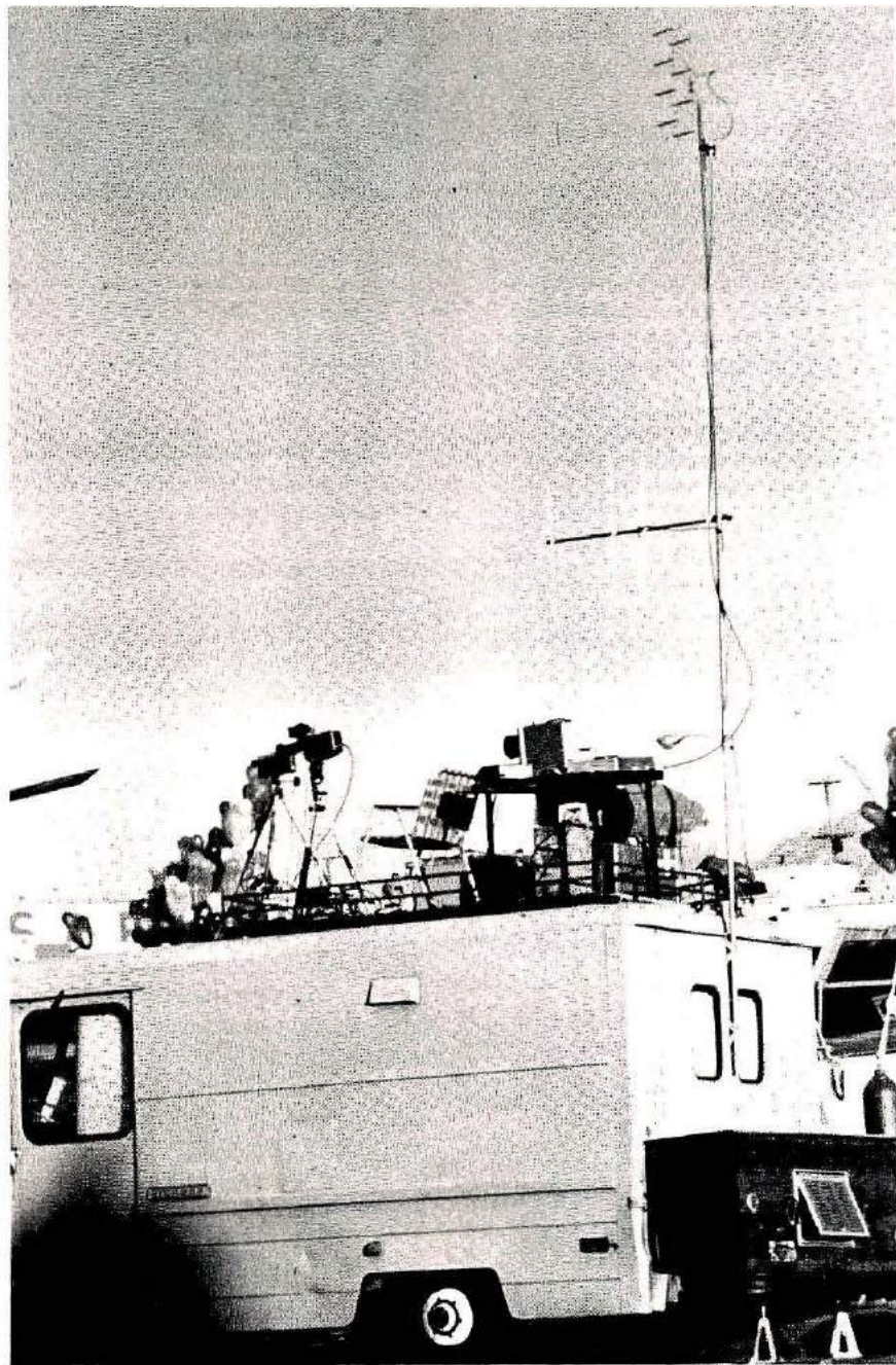
Before the parade, dawn's early light catches the Amateur communications van set up and ready. A two-meter yagi and a collinear array for 420-MHz adorn the mast, and a pair of ATV cameras are ready for their crowd- and float-watching duties. The 1978 Tournament of Roses Parade saw over 70 Amateurs, either on foot or mobile along the parade route, ready to advise parade headquarters of problems, and speed help on its way if needed. The 1979 parade had even more hams helping out, and they plan to do it again in 1980 (photo by K6PGX).
