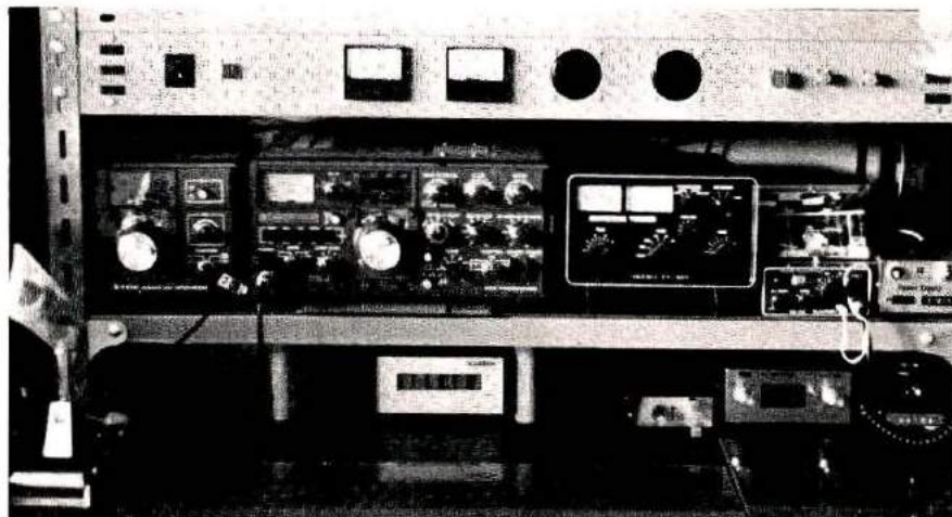
JA1BA uses his TS-820 as the main transceiver, with an earlier TS-510 as a backup. Other parts of his station include some 20 receivers, most of them military surplus!
